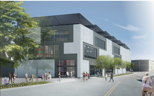
top: The first Behnisch Architekten proposal for Artists for Humanity—a net-zero project in Boston—included a curtain-wall scheme that could not achieve the required U-Value necessary for a net-zero project.
